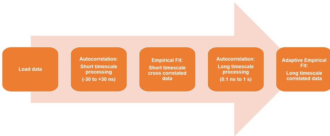
Figure 33: Procedure for Autocorrelation Data Processing and Empirical Fitting
